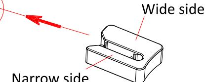
Mount the damping clamp on the louver bracket between louver no. 2 and 3;
