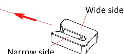
Mount the damping clamp on the louver bracket between louver no. 7 and 8;
